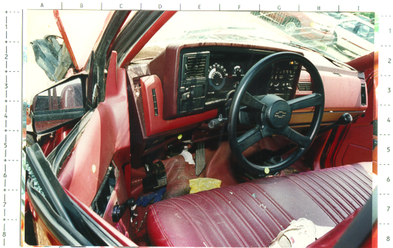
# 81 -- Interior view of driver's area of 1988 Chevrolet pickup; NOTE: contacts (dots) to door panel, steering wheel, & lower dash
